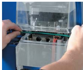
Select job, insert wire or cable.
