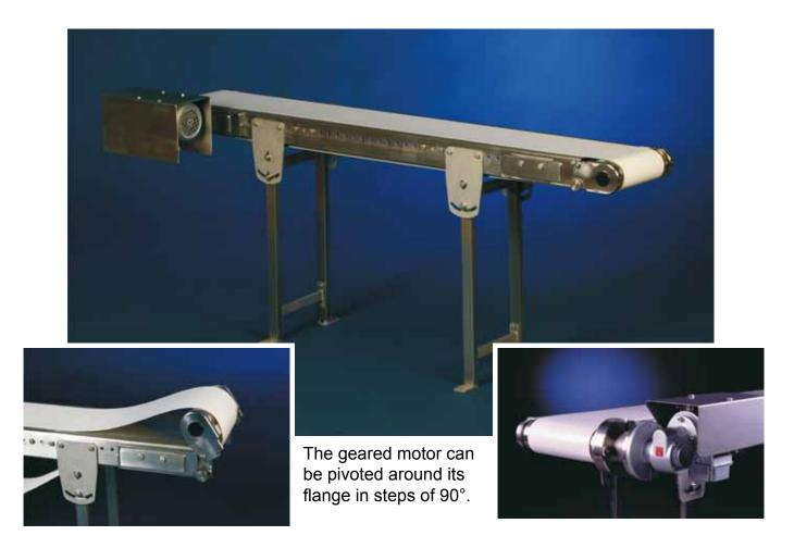
In order to comply to high hygienic standards, the flat belt conveyor GES-80 is equipped with an easy-cleaning mechanism to flip up the deflecting roller.
