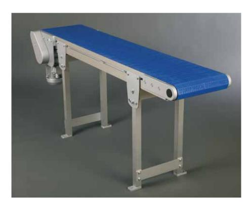
The AM-F with plastic modular chain comes in a very slim design. Thus the frame is only 14 mm wider than the chain. Also at the deflecting roller the brackets add only 40 mm of width. The whole height including the chain is only 95 mm.
