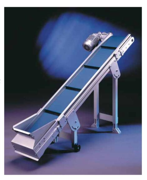
In a standard configuration the GKAL-60 is equipped with a slatted belt, side guide rails and a receiving hopper with fall black flap. The slats on the belt normally are 20, 30 or 40 mm high. But special heights are also available. The distance between the slats on the belt can be freely chosen. The receiving hopper exists in a small and a big standard version. A lot more of the versatile accessories in our program can be found on the pages 69 to 76 in this brochure.
