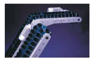
The TorsioDur frame is highly resistant to torsion and has a height of 60 mm. In its grooves along both sides it has sliding blocks with M-8 threads that can be used to fix additional accessories very easily. Therefore the conveyor can be adapted for various applications.
