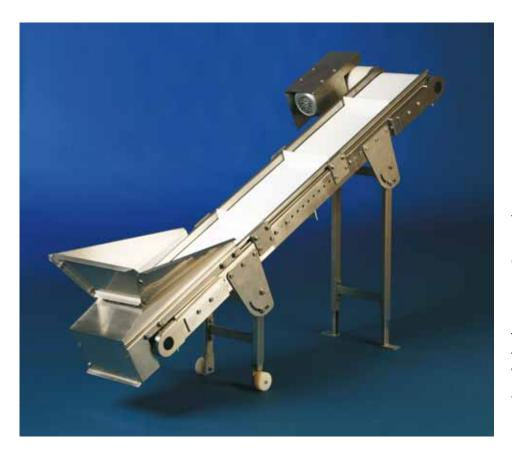
The inclined belt conveyor in stainless steel GKES-80 is equipped with a receiving hopper and it has cross slats on the belt. Along the belt run fixed side rails to guide the transported goods. With these aids it can lift all sorts of bulk and solid material to the required height.
