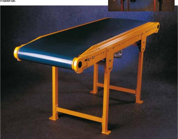
The frame of the GF-80-M is built with 80 mm high steel profiles that are provided with 9 mm holes at 30 mm intervals. Accessories and add-on pieces can be mounted on these holes by using M8 bolts. Hence, the GF-80-M can be easily adapted for various applications.
