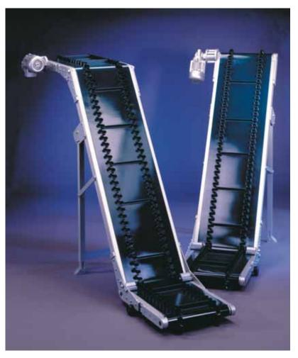
The GAL-Z-W, contrary to the GAL-60-K-W on page 47, has a third section at the upper end of the frame. The transported goods can be fed to a next machine, as though they came from a horizontal conveyor, although they have previously been lifted.
