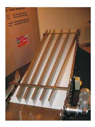
At the end of the belt conveyor is a discharge chute of which angle and position can be freely adjusted.
