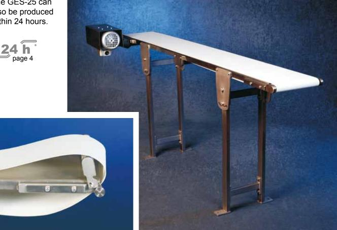
The stainless steel flat belt conveyor GES 25 provides a very hygienic solution for all applications in very confined spaces. With its frame height of only 25 mm and an extremely small deflecting roller diameter of only 30 mm, it is particularly suitable for the transportation of small items. Any length between 500 and 6.000 mm can be produced, simplifying its integration into existing production processes.
