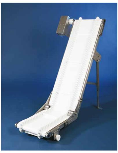
The angle of the rising section can be infinitely adjusted between 40 and 60° from the ground.
